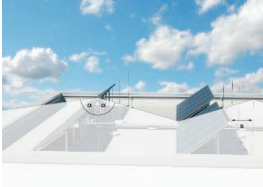
\alpha^\circ = lightning protection angle, s = separating distance
